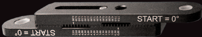
Close-up of the graduated load-bearing bar: it's designed to enable a setting increment of 0.25 degrees in the angle between array elements.
